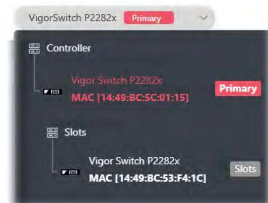
Click **Primary** or **Slots** to open the web user interface of the selected device. A primary device can connect up to three slot devices (via fiber cable).
