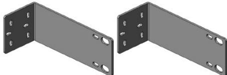
1. Attach the brackets to the chassis of a 19-inch rack. The second bracket attaches the other side of the chassis as above procedure.
